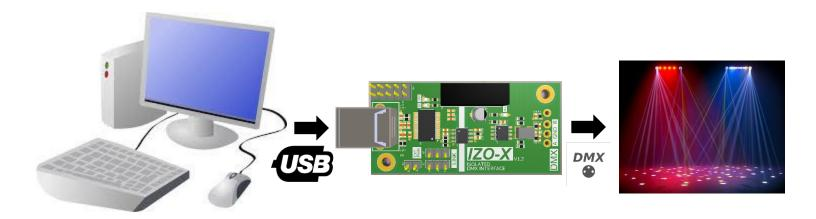
With the IZO-X USB/DMX interface you open the door to professional stage lighting. With a PC application you will easily control a complete universe of DMX lights. The IZO-X interface has an isolated DMX output which means there are no connection whatsoever between the PC and the light fixtures. This gives a clean DMX signal free of ground interference and also provides a safe way to connect your equipment together.
